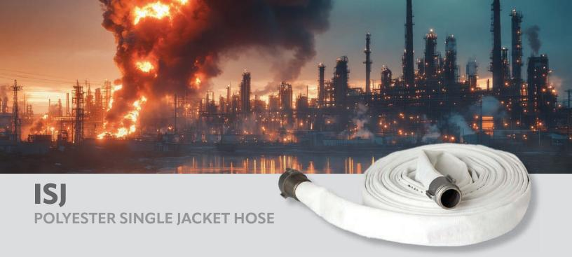
ISJ is a practical choice for a single-jacketed, polyester, EPDM rubber-lined fire hose. It can handle a variety of fluids, including some chemicals and petroleum-based products. With a working pressure of 250 PSI, it features aluminum or brass NH/NPSH threaded couplings and is suitable for general industrial and construction use, mill discharge, in-plant fire protection, and wash down and maintenance tasks.
